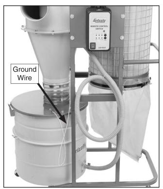
Figure 21. Hose and bag installed.
